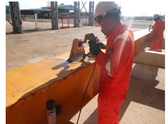
MPI on Padeye Test
