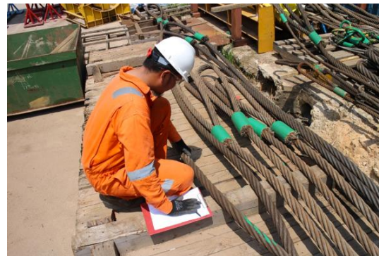
Lifting Gear Inspection
